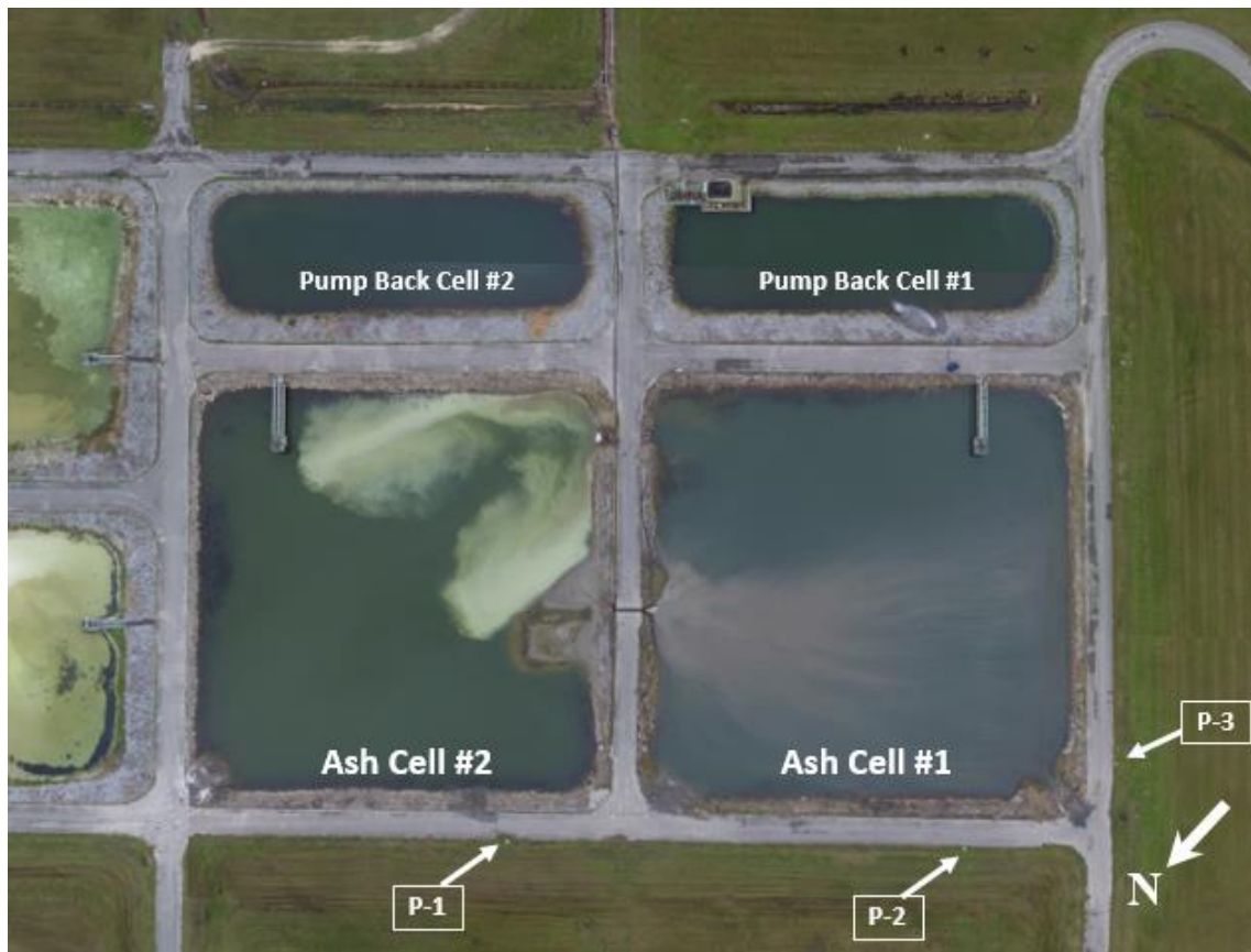
Figure 1. Layout of the CCR Surface Impoundment System and Adjacent Pump Back Ponds (IWCS 2016a)
